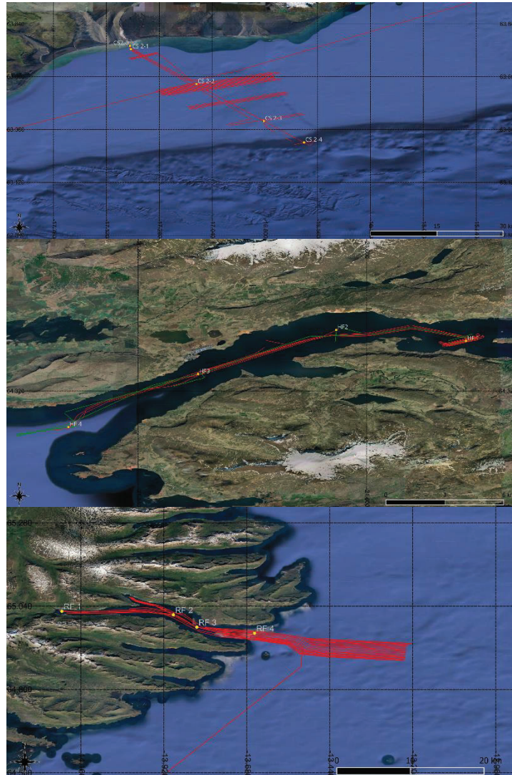
Figure 2: MBES tracks in the shelf area (top), Hvalfjörður (middle) and Reydarfjörður (bottom). Green lines indicate TOPAS subbottom profiler, red lines multibeam echosounder.
